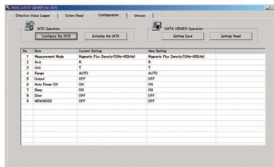
The Magnetic Field HiTESTER 3470 can be set up from the PC application. The settings or measurement conditions are stored on the PC to permit any subsequent downloading that may become necessary
