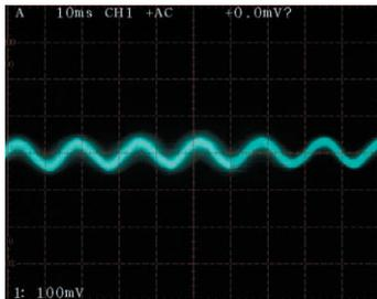
■ Example of waveform measurement using 3471, 60 Hz, 0.1  $\mu\text{T}$  (= 1 mG)
