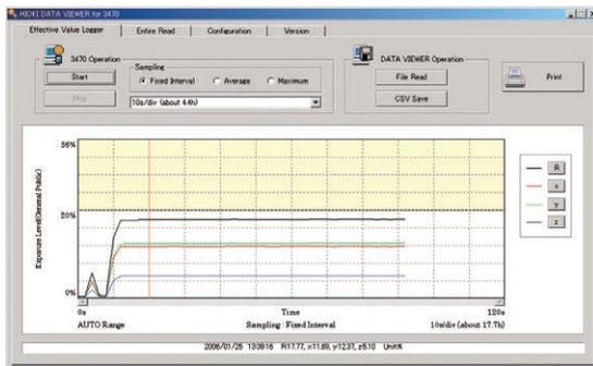
Connect the Magnetic Field HiTESTER 3470 to a PC for extended recordings of measurement data such as tri-axial (x, y, z) and composite (R) RMS values in CSV format. Select from three sampling methods: fixed interval, average and maximum value.
