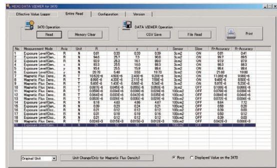
This function enables quick exporting of up to 99 measurement data items stored in the Magnetic Field HiTESTER 3470, a convenient feature when a device must be measured at multiple points.
