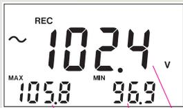
Using the record function, it is possible to check the amplitude of fluctuations.
