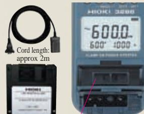
Data output connector RS-232C interface by optical insulating coupler
