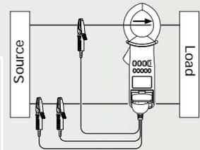
This displays the result of vector calculations on single-phase power.
